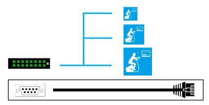
2. Connect serial hub to the Windows computer with USB cable.
